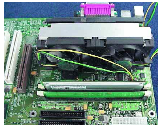
Fig. 1: To avoid trouble, Rambus requires all the RIMM slots to be filled, using a dummy if necessary
