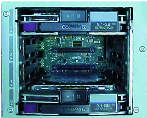
Fig. 3: Special cartridges are used to allow drives to be hot-swapped
