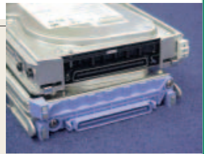
Normally the SCA connector is found only in OEM systems and module recognition is done optically.
