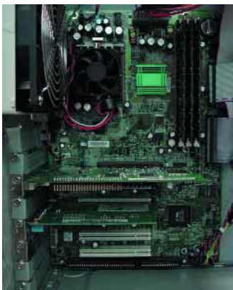
The main board runs at a frequency of 133 MHz.
