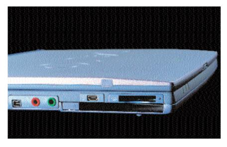
The price of compactness – there is only one CardBus slot available which is already taken up with connecting the CD-ROM. the back right-hand corner where the modem lead is inserted at an angle of 45 degrees.
