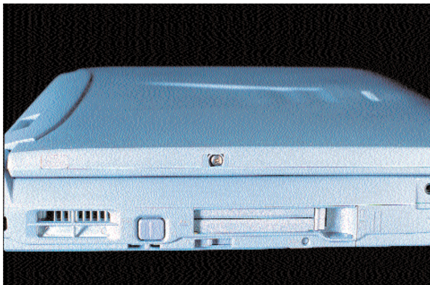
Not quite so obvious is the little catch under the switch on the Satellite Pro 4300.
