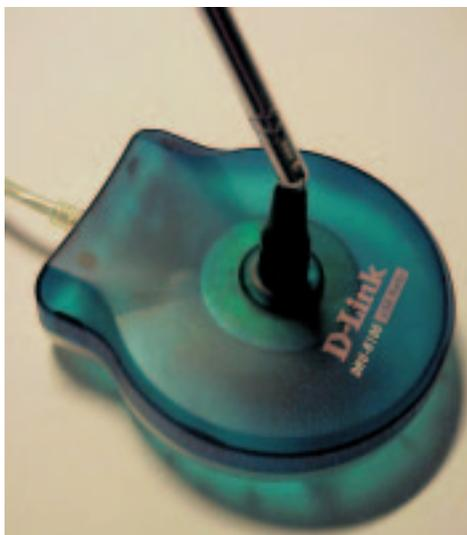
With the D-Link DRU-R100 Radio only the frequency can be adjusted by USB. The sound has to be tapped by analogue means
