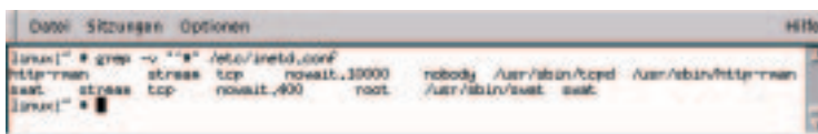
Figure 3: Almost all utilities were superfluous: we need http-rman for the SuSE help system, swat stands in for the system administration program linuxconf of other distributions.
