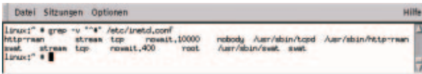
Figure 3: Almost all utilities were superfluous: we need http-rman for the SuSE help system, swat stands in for the system administration program linuxconf of other distributions.
