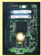
replacing the stylus in the PDA also turns it on and off. Nevertheless, the batteries do not last particularly long and were run flat after a week's intensive use. Agenda would have perhaps been better to select the AA size batteries, which are not much larger, but have almost three times the capacity.
