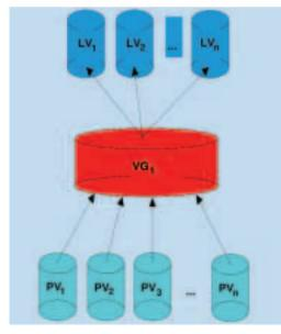
Figure 1: The three-level memory architecture of the Linux LVM
