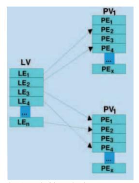
Figure 2: Example of the mapping of an LV onto two different PVs
