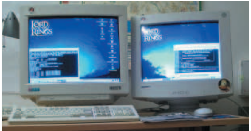
Two desktops from one machine. Both have a KDE panel but only one has desktop icons
