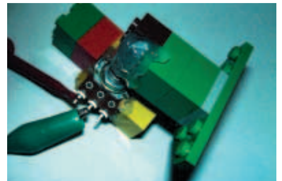
Hot glue – the quick fix solution. Angle sensor using a potentiometer
