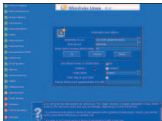
The 'Install bootloader' section in Mandrake. To stop your existing bootloader from being tampered with change the 'boot device' to /dev/fd0
