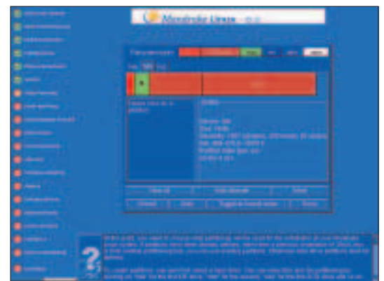
Here are the partitions set aside for the new install. You only need a '/'. You don't need a separate '/boot' or 'swap space' – learn by my mistake
