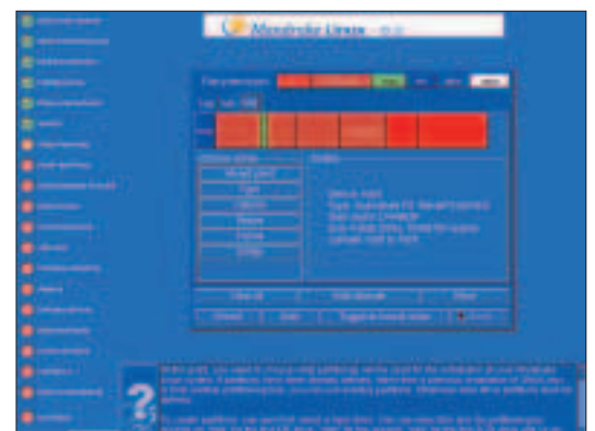
Here you can see how I have mounted my original '/home' partition in the new installation, giving it the name '/mnt/home2'
