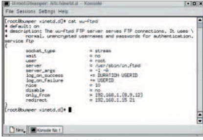
Figure 3. Redirect entry in the FTP (wu-ftpd) file
