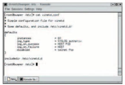
Figure 2: Listing of /etc/xinetd.conf with FTP and Telnet disabled
