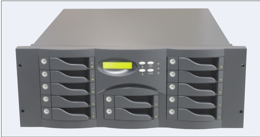
Figure 1: Two node failover cluster configurations require a dual channel SCSI RAID or fiberchannel solution that can be accessed simultaneously by both nodes.
