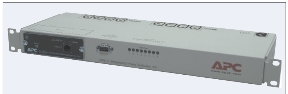
Figure 2: The Master Switch AP9212 can switch eight power circuits individually. The integrated web server provides administrator access to the management software via SNMP or telnet.
