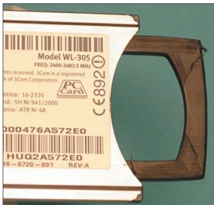
Figure 1: Cigar cutter included: The upper and lower halves of the lid are so sharp that they strip the plastic coating off the antenna – you can plainly see the plastic shavings and cuts
