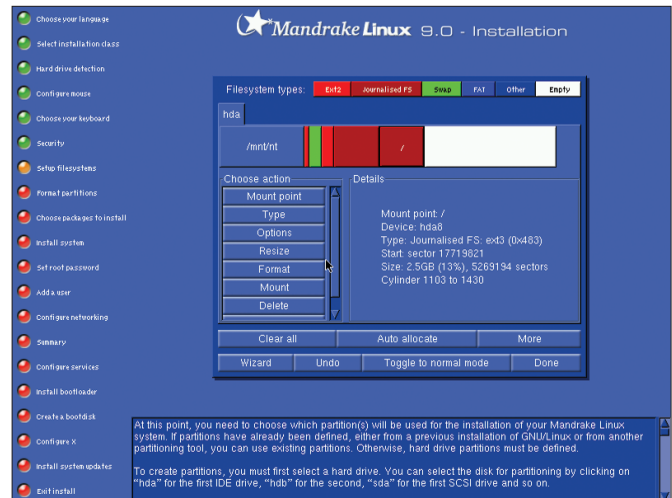
Figure 2: Mandrake is installed on /dev/hda8 and merely uses /dev/hda5 as a swap partition. The partitions for /boot and /home will be merged manually after installing
