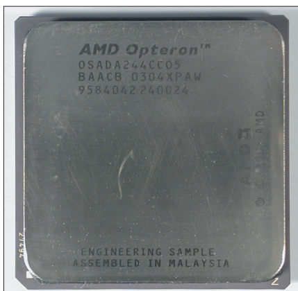
Figure 3: The 1.8 GHz CPUs were pre-production engineering samples
