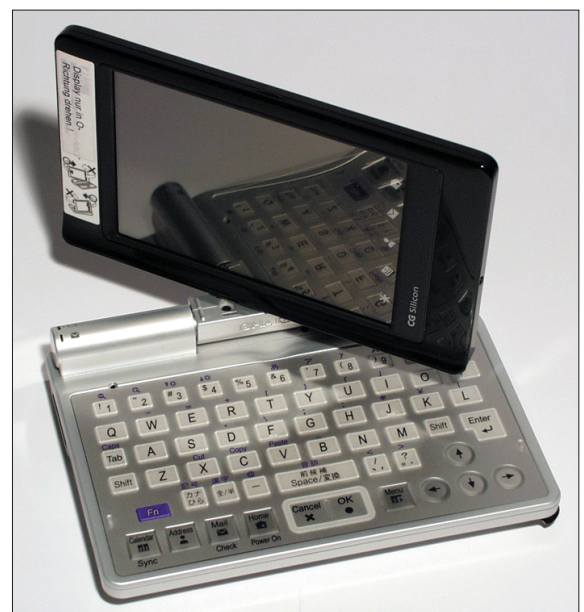
Figure 3: The high resolution display – 640 x 480 pixels at 200 DPI – of Sharp's Zaurus can be rotated through 90 degrees on its hinge
