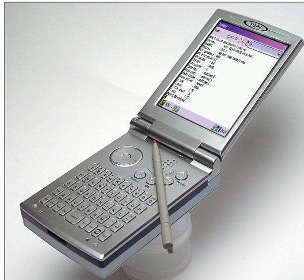
Figure 5: Yopy YP-3500 is small and feels good in the hand, though it is somewhat chunky with its Compact Flash slot behind the display hinge
