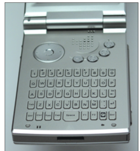
Figure 1: The keyboard of the new Yopy YP-3500 and YP3700 has the standard QWERTY layout, which makes for very small keys
