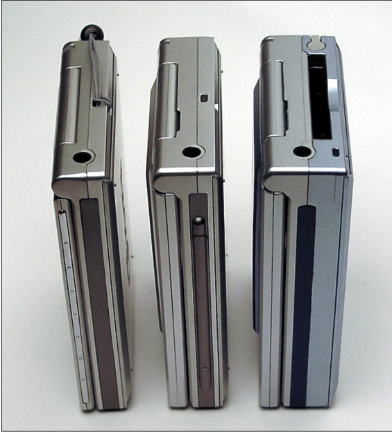
Figure 2: The Yopy YP-3500 (center) is 2cm thick (3/4 in), much thicker than the YP-3000 (left). And with the Compact Flash slot, the YP3700 is just under 2.5 cm (1 in) thick
