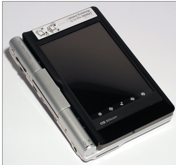
Figure 4: The Zaurus as a complete pen PDA for single handed use. The desktop software automatically rotates 90 degrees
