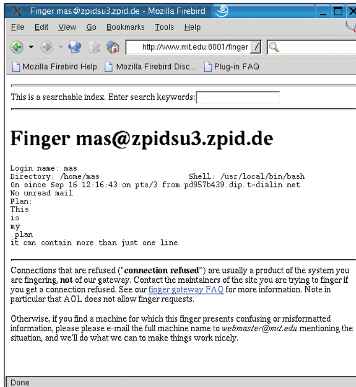
Figure 1: If you want to add a finger request to your homepage, you can use a Web interface to do so. As the protocol is extremely simple, it does not take long to develop a front-end
