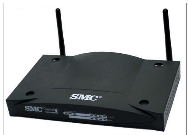
Figure 2: The SMC2804WBR Wireless Access Router includes an internal switch with four Ethernet ports, and a 10/100 Mbit Ethernet port for DSL or network attachment. The firmware provides both packet filtering and a firewall, and a Web front-end for administration tasks
