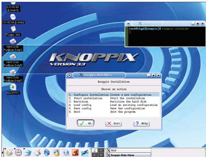
Figure 1: The knoppix-installer script launches a GUI-based installer, allowing you to copy the original Knoppix from CD and install it on your hard disk.
