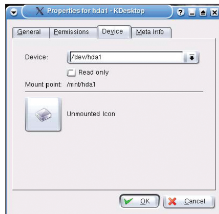
Figure 3: Use the KDE desktop to enable write access to both partitions, as Knoppix tends to prefer mounting with read-only access.
