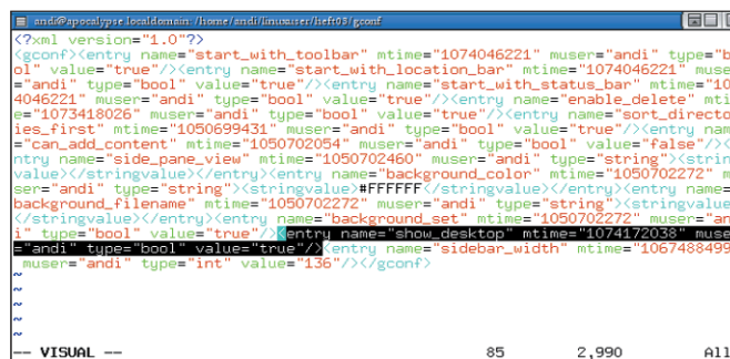
Figure 3: Gnome uses XML files of this kind to store its configuration data.
