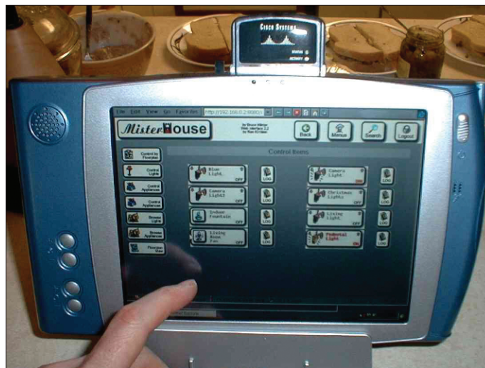
Figure 1: Mister House, the software for the intelligent house. Use a Web browser to control any device in your home. A handheld computer like the Aquapad is highly recommended.
