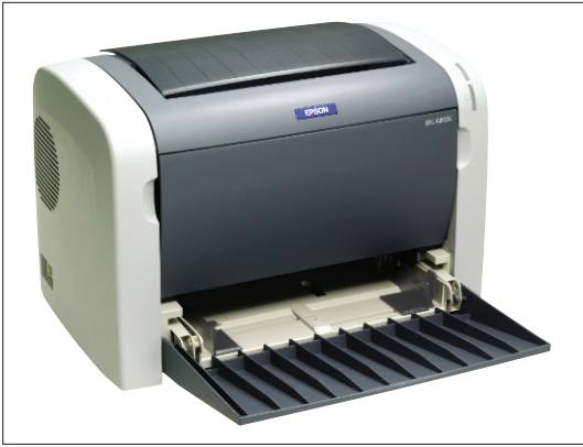
Figure 4: Linux support is questionable for low-budget Epson laser printers. The Epson EPL6200L only has partial support as it uses a proprietary protocol.
