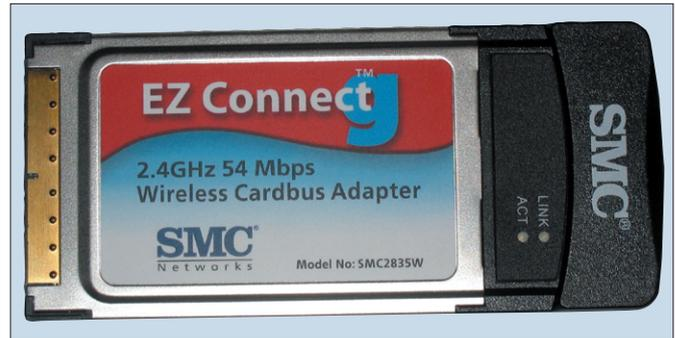
**Figure 3:** 54 Mbit WLAN cards like this SMC2835W with a Prism chipset are quite widespread nowadays, and not much more expensive than their 11 Mbit predecessors. Thanks to Mad Wifi and Prism 54 most of them now work on Linux.
