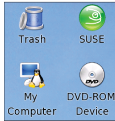
Figure 6: The device icon bottom right shows that the DVD is not mounted.
