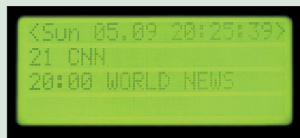
Figure 1: LCDproc displaying the channel name on the LCD attached to my digital video recorder.
