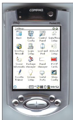
Figure 1: This HP/Compaq iPAQ runs Linux now instead of the preinstalled version of Windows Mobile.
