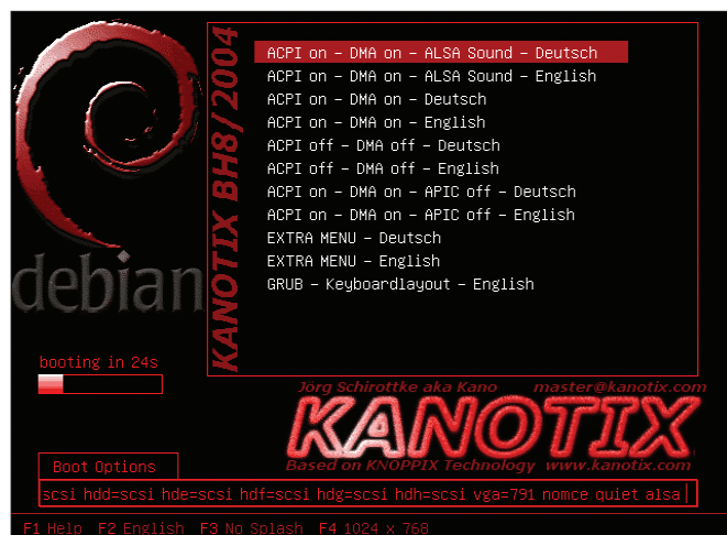
Figure 1: In contrast to Knoppix, Kanotix has a GUI-based boot menu where users can select cheat codes.
