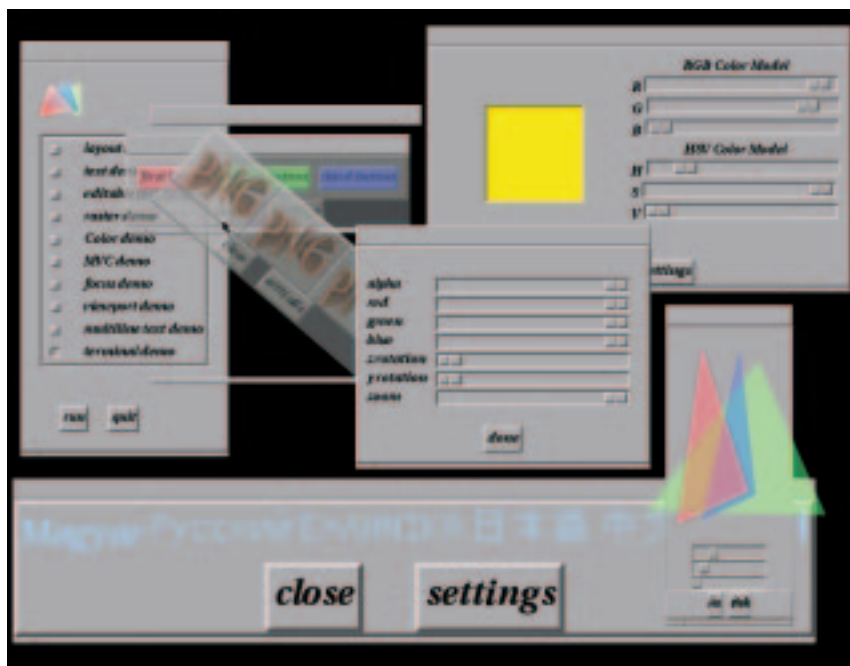
Fig. 1: Whether rotated or enlarged: TrueType- and Bitmap fonts are improved in quality as the result of edge smoothing.
